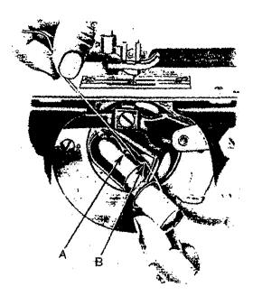
Fig.4 Bobbin Replacement and Threading the Shuttle
