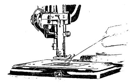
Fig. 8 Drawing up the Bobbin Thread
