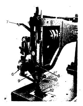
Fig.7 Threading the Needle
