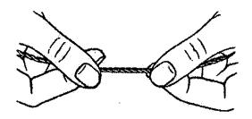
Fig.1 How to determine the twist Hold the thread as shown in Fig.1 .Turn the thread over toward you between the thumb and forefinger of the right hand.If left twist, the strands will wing tighter.If right twist, the strands will unravel.
